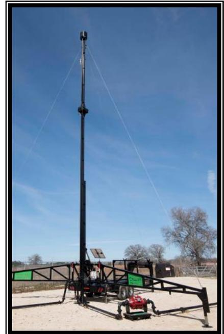
Trailer mounted flare stack –60 feet dual stack (6" & 3") unit
